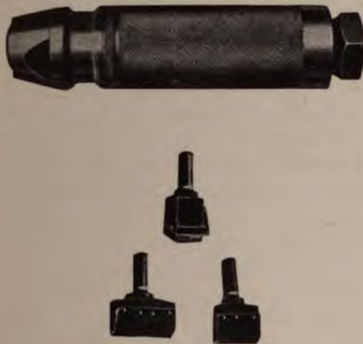
FIG. 50.—The author's pneumatic hammer with concussors.
